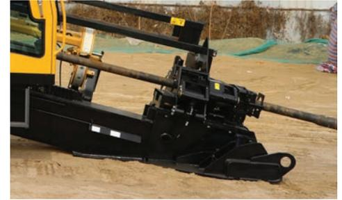
**OPTIONAL FRONT-MOUNTED STAKEDOWN SYSTEM.** Helps reduce the amount of time and materials needed to set up and secure the drill for enhanced jobsite efficiency.
