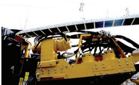
**THREE-SPEED GEARBOX.** Helps improve the overall drilling efficiency by allowing the operator to adjust the machine's rotational torque to match different ground conditions.
