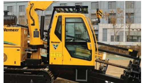
**CLIMATE-CONTROLLED CAB.** Enhances operator comfort and provides protection from the weather, which reduces operator fatigue and discomfort, helping you be more productive.
