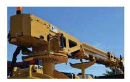
HYDRAULIC BOOM (OPTIONAL). Exclusive telescoping boom maintains hose length during extension and incorporates a remote-controlled hydraulic valve for vacuum shutoff. Available with manual or hydraulic rotation.
