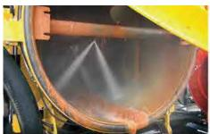
IN-TANK WASHDOWN. Delivers a high-pressure water spray to the tank interior helping to simultaneously dump material and clean the inside of the tank. Saves cleanup time and makes it efficient to remove difficult debris.
