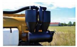
THREE-STAGE CYCLONIC FILTRATION. Engineered to help prolong filter and blower life, the system is suitable for wet and dry applications. The cyclones use a tuned vortex system in which the outer vortex spiral forces small particles to fall into a separate canister. The filtered stream then passes up through the inner cyclone tube and is carried to the final poly filter.
