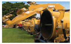
CAM-OVER REAR DOOR. Provides a 360-degree positive seal, even under reverse pressure without additional clamping requirements. The highly reliable cam-over door has no in-tank moving parts, so all maintenance is external.
