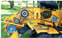
**CONVENIENT BELT SERVICING.** Belts on the SC292 are serviceable from one side of the machine with cutter drive belts being adjustable with movable idlers. Additionally, each belt set may be adjusted independently, without affecting adjustment of other belts.
