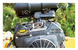
START EASIER. Equipped with a 26.5 hp (19.8 kW) EFI Kohler engine, the SC292 performs well in cold-weather starts, has reduced occurrence of engine flooding and provides improved fuel economy over comparable carbureted gas engines.
