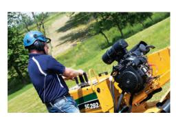
TWO-SPEED GROUND DRIVE. The operator may choose to operate in a high-range or low-range ground speed setting of 0-133 fpm (0-40.5 m/min) to quickly move the machine or choose a slower speed when near the stump by utilizing a low-range setting of 0-66 fpm (0-20.1 m/min).
