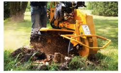
AUTOSWEEP® CONTROL SYSTEM. When equipped, the AutoSweep system monitors engine speed and automatically adjusts cutter wheel sweep rate, and is designed to reduce engine, drivetrain and structural stress.
