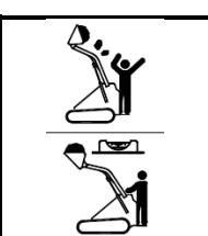
**WARNING:** Falling load can crush.
