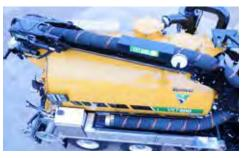
**TSUNAMI ULTRALIGHT BOOM.** This 8-in (20.3-cm) boom is constructed out of strenx performance steel making it lighter than a traditional unit.
