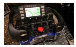
**IFM ELECTRONICS.** Industry leading IFM industrial controller that monitors the systems temperature, pressure and vacuum sensors. It also allows the operator to see the engine instruments, the chassis instruments, as well as the vac instruments on the belly pack.
