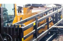
The cabin offers ideal visibility and spacious work area for the operator to work in a variety of climate conditions. Dashboard controls are lined with the vice and entry pit and large windows provide clear visibility of the rack, vices and borepath.
