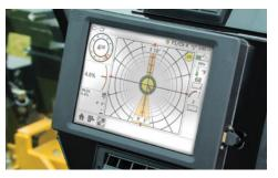
AURORA<sup>™</sup> TOUCHSCREEN DISPLAY. Interactive, full-color display provides real-time location information plus tools to complete drilling activities more efficiently, and can replace the need for hard copy bore plans.
