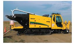
**IMPRESSIVE SIZE-TO-POWER RATIO.** The D60x90 S3 boasts up to 60,000 lb (267 kN) thrust/pullback and 9,000 ft-lb (12,202.4 Nm) of rotational torque at just 100" (254 cm) wide and 26' long (7.9 m), so it's qualified for a range of installation specifications even in congested urban jobsites.
