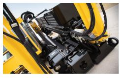
**LARGE OPEN-TOP VISE DESIGN.** The D60x90 S3 features a large open-top vise design for the purpose of removing and adding tooling.
