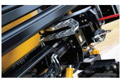
**CONVENIENT ROD LOADING.** Easy-to-operate and reliable rod loader is inspired by the popular and proven D24x40 Series II design.
