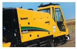
**INCREASED POWER.** The D60x90 S3 boasts a sizeable 17 hp (12.7 kW) increase over its predecessor, the D60x90, giving operators more power for drilling in difficult ground conditions.
