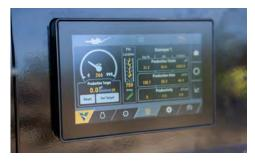
**EFFICIENCY MADE SIMPLE.** The optional Vermeer productivity monitoring system provides real-time data on machine performance and allows you to track the volume of material processed by visualizing cubic yards per gallon of fuel.
