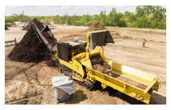
**COLORING MADE EASY.** The optioinal Vermeer coloring system, fully integrated into the grinder, reduces the number of machines required and minimizes handling of material, adding value to your end product. This system optimizes dye and water usage, minimizing your cost per yard.
