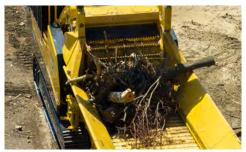
POWERFUL FEEDING. With a feed opening of 60 in x 30 -in (152.4 cm x 76.2) and robust infeed sidewalls that are double the strength of its predecessor, you can feed whole trees and other large material with less restriction. The machine sidewalls also provide optimal flow of material and minimize operator interaction.
