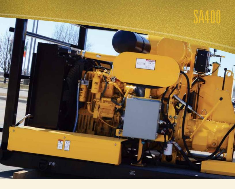
A triplex piston pump produces up to 550 gpm (2082 L/min), providing a continuous flow of drilling fluid during drill operations.
