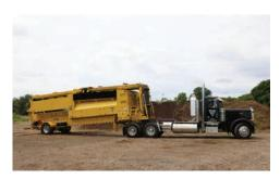
TRAILER MOUNTED. Machine is mounted on a trailer to promote ease of mobility to and from the jobsite as well as on the job.
