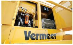
**ELECTRIC MOTOR.** This machine is powered by an industrial-duty, fully enclosed and fan-cooled electric motor. A single 60-hp (44.7-kW) motor powers the hydraulic pump stack. The electric motor has lower exhaust emissions, jobsite noise and maintenance compared to diesel.
