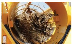
TENSION SCREEN DESIGN. The tension screen design allows the operator to change screen opening size, wire gauge and type of wire to allow for separating a wide variety of material. Operators can quickly change screen sizes by five large bolts adjusted by the tensioning hook.
