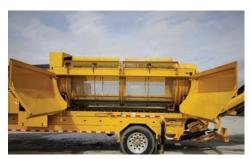
**ACCESS TO CRITICAL POINTS. Perform** machine maintenance efficiently through ease of access to components such as motor, trommel drum and drum drive.
