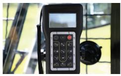
ADVANCED CONTROLS. This machine features a live time display remote. Operator can adjust drum speed, hopper feed, conveyor feed and height adjustments via the transceiver remote.
