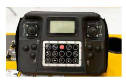
OPTIONAL REMOTE CONTROL. The SC402 is remote-ready - putting control back in your hands. This provides operators with the flexibility to maneuver the machine and grind stumps comfortably on diverse jobsites.
