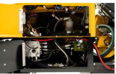
EASE OF MAINTENANCE. Designed for ease of maintenance, the SC402 is all about access and convenience - helping you spend less time in the shop and more time in the field grinding.
