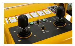
**OPERATOR PRESENCE SYSTEM.** The SC402 features the safety innovations you've come to expect from Vermeer - like the capacitive-sensing operator presence system that disengages the wheel when your hands leave the controls.
