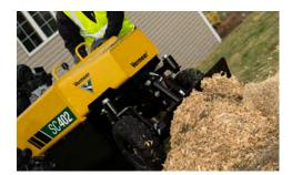
OPTIONAL BACKFILL BLADE. When it's time to clean up at the stump, the SC402 was engineered to maximize the containment of chips and get them back in the ground quickly thanks to the optional hydraulic backfill blade.
