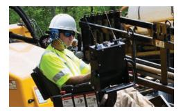
**SIGNIFICANT SOUND REDUCTION.** With a 104 dB(A) guaranteed sound power level and an operator ear rating of 82.9 dB(A) [in-cab rating of 75.7 dB(A)], the D40x55 S3 is significantly quieter than its predecessor – contributing to a quieter working environment with less neighborhood disturbance and easier communication among the crew.
