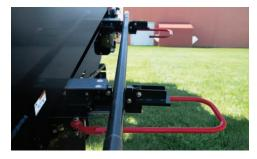
**VARIETY OF ROD OPTIONS.** The D40x55 S3 is available with a range of drill rod options, including a 10 ft (3 m) length in 2.38 in (6 cm) or a 2.63 in (6.7 cm) diameter, and a 15 ft (4.6 m) length in a 2.63 in (6.7 cm) diameter. A variety of rod options allows the drill to be configured to the specific needs of the contractor.
