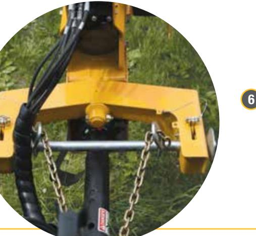
**6** A patented 2-point Quick Hitch hookup is designed to allow one person to hook up the mower. It also provides high ground clearance to help avoid obstructions while in the field.
