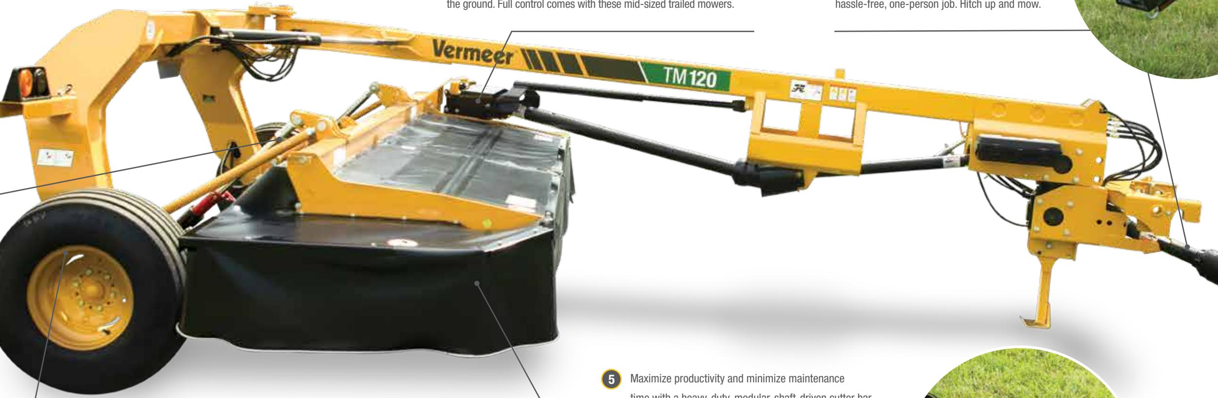
**5** Maximize productivity and minimize maintenance time with a heavy-duty, modular, shaft-driven cutter bar. Not only is it backed by the Vermeer 3-year cutter bar coverage, but two features make it quick and convenient to replace key components — the Quick-Clip<sup>®</sup> blade retention system and Quick-Change<sup>TM</sup> shear ring. Get back up and mowing in the field.
