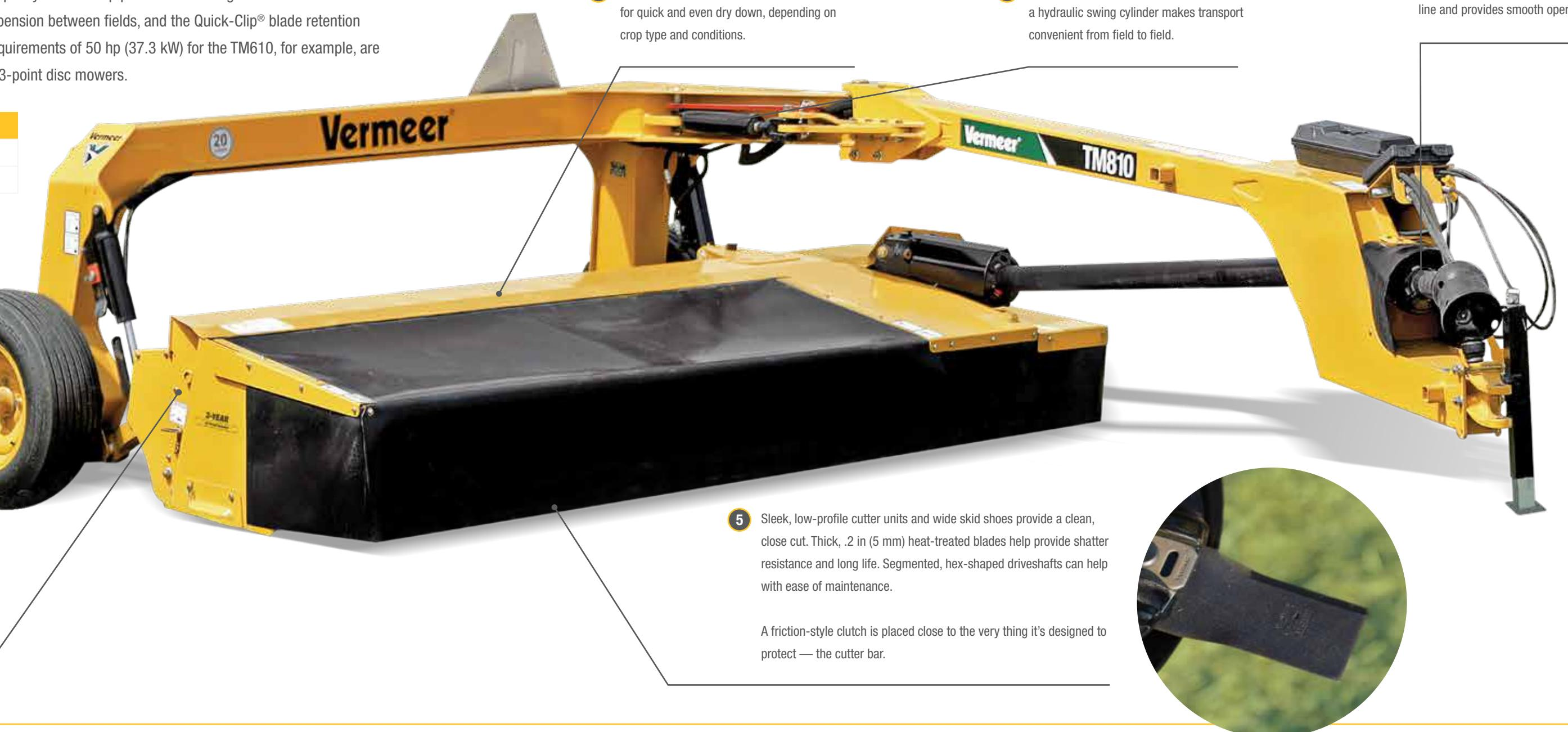
**1** An exclusive rubber torsion suspension design absorbs shock loads and high impacts by reducing cutter bar weight on the ground, allowing it to float and swing up and over field obstacles.
