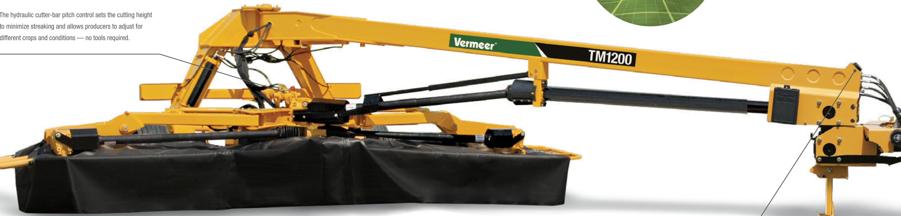
**4** Float over fields and contoured terrain with a nitrogen-charged accumulator flotation system that adjusts for varying field and crop conditions.
