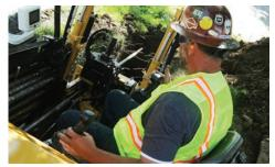
LOW SOUND LEVELS. Low noise emission levels at the operator's ear of 85 dBa and a guaranteed sound power of 104 dBa make this drill perfect for installing small utilities in an urban environment with minimal disruption.
