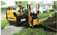
NARROW FOOTPRINT. This drill is 8.5 in (21.6 cm) narrower in width than the next sized drill in the lineup and can get through a 36 in (91.4 cm) gate or fit on a narrow trailer with other jobsite essentials.
