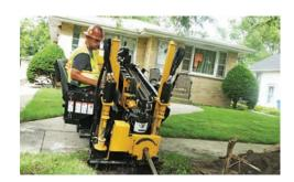
MORE POWER. Equipped with a 48 hp (35.8 kW) Rehlko engine, this drill offers 1,200 ft-lb (1,627 Nm) of spindle torque and 7,850 lb (3,563.9 kg) of thrust/pullback.
