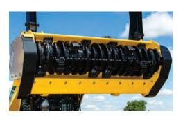
**ABOVE-GROUND MULCHER - RINGED** ROTOR. The ringed rotor design of the aboveground mulcher head attachment helps guide material into the path of the cutting tips for effective single-pass clearing and full-tip coverage. By controlling the depth of cut, the engine can be loaded to peak operating performance.
