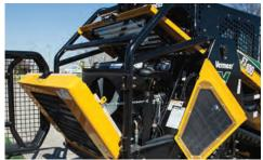
**ENGINE ENCLOSURE.** Engine compartment doors provide convenient access to maintenance points.
