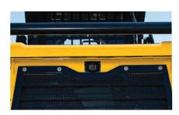
**REAR CAMERA WITH IN-CAB MONITOR.** An in-cab monitor provides added visibility, enhancing maneuverability.
