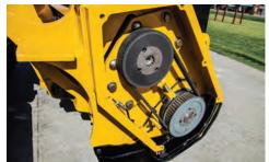
SYNCHRONOUS BELT DRIVE. This compact design enables the overall width of the mulcher head to remain narrow enough to work in tight places. In addition, the driveline is easily accessible for maintenance.
