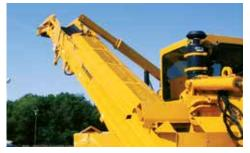
**OPTIONAL LOADING CONVEYOR.** An optional stowable loading conveyor stores easily, and unlike competitive models does not require removal for transportation.
