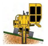
**OPTIONAL AUTO TILT TRACK.** An oscillating track frame allows the track to follow the ground's contour providing a vertical trench on slopes up to 10 degrees.
