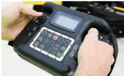
**OPTIONAL REMOTE CONTROL.** An optional remote control allows operators to maneuver the stump cutter while away from the unit.
