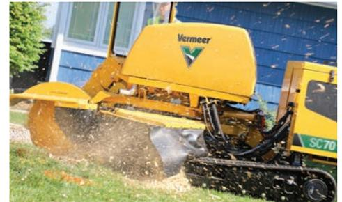
**PRODUCTIVE CHIPPING.** With a 67 hp (50 kW) Cat C2.2L turbocharged Tier 4 Final/Stage V diesel engine, this machine is ready for tough cutting jobs.
