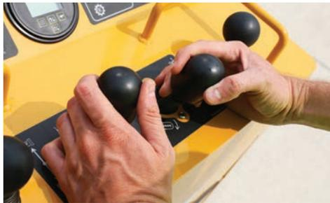
**OPERATOR PRESENCE SYSTEM.** This operator system is intended to help protect the operator. If the operator's hand(s) leave the cutter wheel controls for more than one second, the cutter wheel will disengage, come to a stop and the cutter wheel indicator light will go out.
