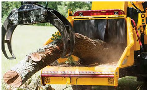
**POWERFUL PERFORMANCE.** Equipped with up to 11,674 lb (5295.2 kg) of pull-in force, this unit has optimized efficiency while working in tandem with the patented SmartFeed system to increase productivity when chipping large diameter logs.
