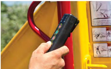
**OPERATOR CONTROL.** The Tree Commander™ remote control comes standard with the AX19, and an optional full-function remote is available. The operator is able to control the functions of the brush chipper remotely to improve jobsite productivity.
