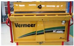
THE PATENTED SMARTFEED SYSTEM. Maximizes operator productivity while reducing strain on vital equipment components. The feed-sensing control system monitors motor current and automatically stops or reverses the feed when feeding large, hardwood material.
