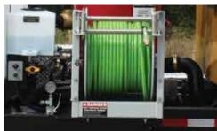
**JETTER REEL.** 15 gpm (57 L/min) @ 1,500 psi water pump with 300 ft x 1/2 in (91 m x 1 cm) jetter hose.
