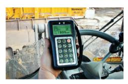
**REMOTE CONTROL.** Discharge height, along with several other machine functions, is adjustable via remote control.
