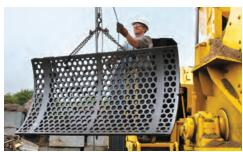
SIMPLE SCREEN CHANGES. Operators can change product sizes easily with the onboard screen handler system.
