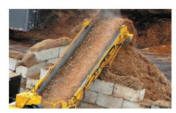
HIGH PRODUCTION. Yield higher volumes of wood waste and reduce spillage or plugging due to a 66" (167.6 cm) wide loadout conveyor, with a discharge height of 14' to 18' (4.3 m to 5.5 m).
