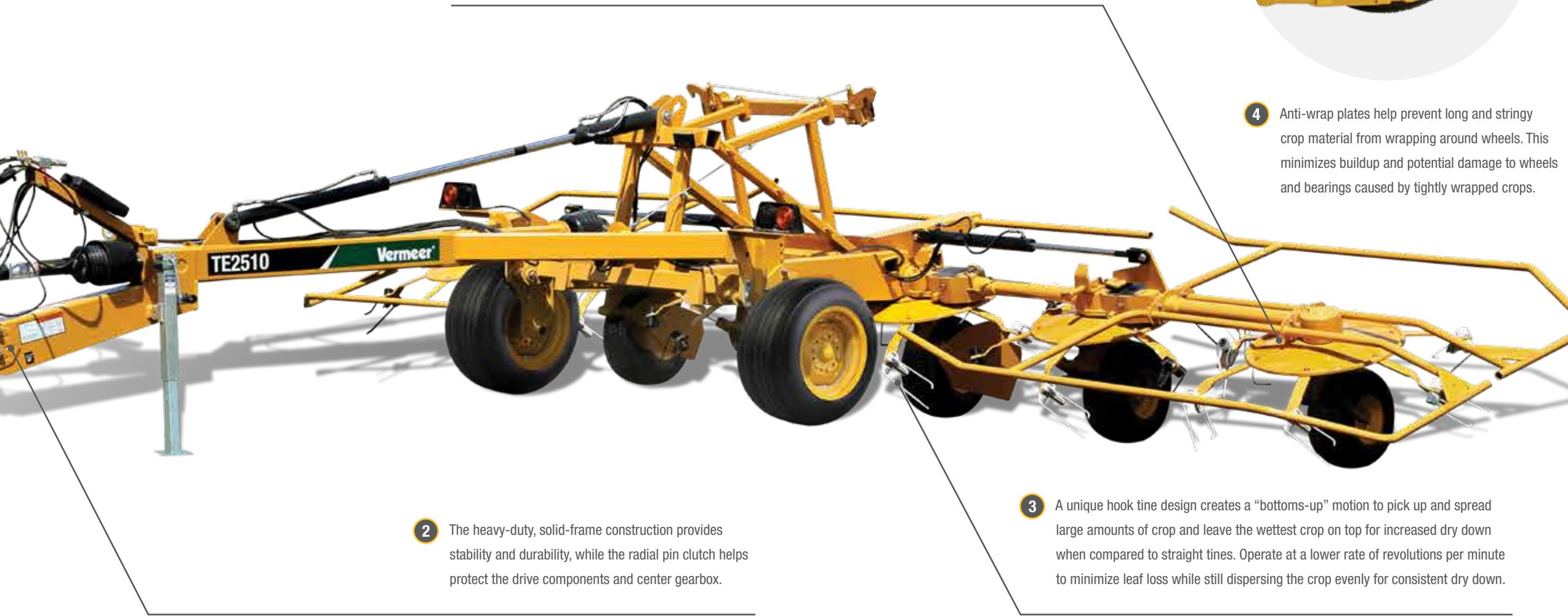
**2** The heavy-duty, solid-frame construction provides stability and durability, while the radial pin clutch helps protect the drive components and center gearbox.
