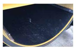
POLYMER LINER. The polymer liner inside the debris tank on the bottom half makes for efficient dumping and cleanout.
