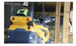
**COMPACT SIZE.** With narrow tires, the ATX720 is 44.5-in (113-cm) wide, while the wider tires make the machine 50.4-in (128-cm) wide. The standard tire configuration allows the ATX720 to fit through a standard 4-ft (1-m) gate for backyard access on landscape jobs.
