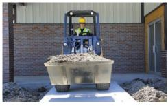
LIFT-CAPACITY-TO-WEIGHT RATIO. The ATX720 has a rated operating capacity of 1,939 lb (880 kg) while having a standard weight of 3,911 lb (1,774 kg). This lift-capacity-to-weight ratio allows contractors to use a light machine while still being able to carry heavy materials on the jobsite.
