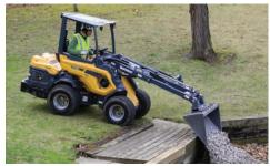
TELESCOPIC BOOM. The telescopic boom on the ATX720 extends 29.1 in (73.9 cm) for loading materials to a dump height of 114 in (290 cm) in hinge pin height. The telescopic boom can also aid in dumping material over the back of a retaining wall or grabbing material over an obstruction.
