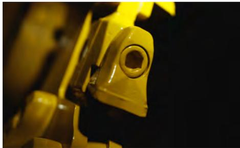
**EASE OF MAINTENANCE.** With convenient features such as a single bolt for all teeth, the system only requires two tooth parts numbers and no other wear parts to maintain. And once torqued, the bolts remain tight until the teeth are removed or flipped.
