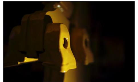
**MINIMIZED RECIRCULATION.** The new wheel design and placement of the teeth allow for material to flow efficiently past the wheel after being cut, minimizing the recirculation of material.
