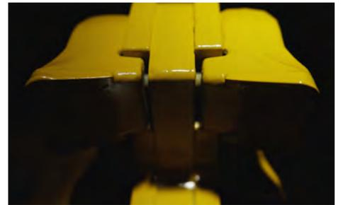
**DOUBLE-SIDED.** The two cutting edges on the VCS tooth provide the operator an advantage over comparable cutting systems.
