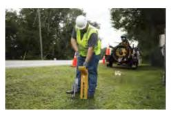
**CURRENT DIRECTION.** Identify target line in congested areas by determining the direction of current flow against "adjacent signals" caused by returning current.
