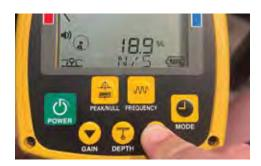
**AMBIENT NOISE DETECTION (A.N.D.).** Helps improve accuracy of locates by determining the frequency with the least amount of interference on your jobsite.
