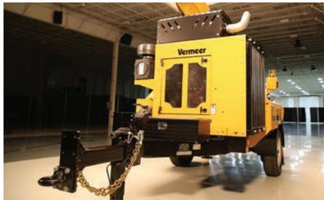
**TRANSPORT FRIENDLY.** The fully configured AX17 is under 10,000 lb (4,536 kg) helps with ease of transportation around congested urban areas and minimizes the need for additional license requirements.
