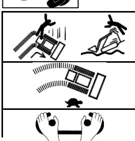
**WARNING:** Abrupt movement and uneven terrain can throw operator off machine.Avoid abrupt starts,
