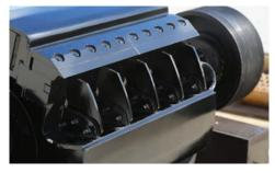
**OPTIMAL CUTTING PERFORMANCE.** Two knife options, with depths of cut of 3/8 in (1 cm) or 5/8 in (1.6 cm), allow the operator to select the knife that meets their end-product sizing needs.
