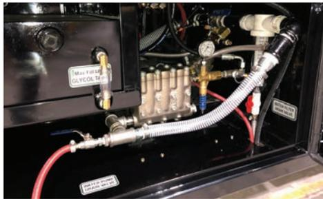
**WATER SYSTEM.** The water system is rated for 19.4 gpm @ 3,000 psi (73.4 L/min @ 20,684 kPa).
