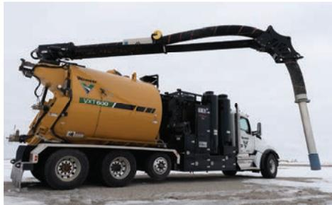
**TSUNAMI ULTRALIGHT BOOM.** This 8-in (20.3-cm) boom is constructed out of strenx performance steel making it lighter than a traditional unit.
