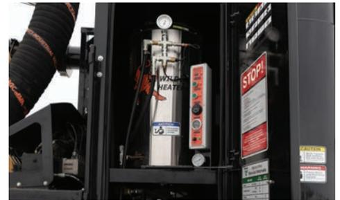
**BOILER.** 420K BTU diesel fired boiler with coils rated at 5,000 psi (34,473 kPa).
