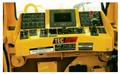
**SMARTTEC ELECTRONIC CONTROL SYSTEM.** SmartTEC performance software helps optimize productivity with real-time machine control prompts. Monitor and record functions encourage proactive machine maintenance and operator performance analysis. Available on all Vermeer TEC<sup>®</sup> Plus computer-aided control system-equipped machines.
