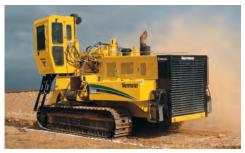
**ELEVATING ROPM CAB.** The elevating rollover protective module cab features LEXAN glass, filtered and pressurized air, heating and air-conditioning. The cab's vantage point allows a virtually unrestricted view of the boom, trench and conveyor.
