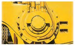
**ROTARY POWER TRENCHER DRIVE MOTOR.** A rotary power trencher drive motor and splined headshaft produce low-speed and high torque which provide superior ground penetration and low chain wear for better production results.
