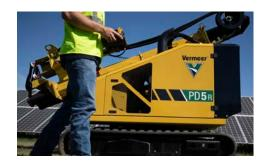
**COMPACT DESIGN.** A small machine with transport dimensions of 85 in (215.9 cm) wide, 8.2 ft (2.5 m) tall and a 15 ft (4.6 m) mast is ideal for jobsites with less space, or for multiple smaller iobs that require continual transportation of the machine. Quickly move around the jobsite and continue efficiency of installations, helping reduce time spent on setup, teardown and transportation.
