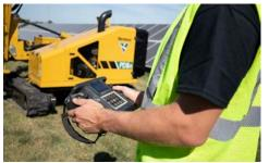
**TAKE CONTROL.** With a wireless remote, crews can operate the PD5R and gain visibility around the machine, while controlling most machine functions like hammer engagement, pile accuracy, auto plumb and ground drive, all while remaining out of an operator's seat during installation.
