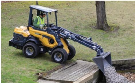
**TELESCOPIC BOOM.** The telescopic boom on the ATX720 extends 29.1 in (73.9 cm) for loading materials to a dump height of 114 in (289.6 cm) in hinge pin height. The telescopic boom can also aid in dumping material over the back of a retaining wall or grabbing material over an obstruction.
