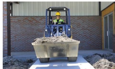
**LIFT-CAPACITY-TO-WEIGHT RATIO.** The ATX720 has a rated operating capacity of 2,155 lb (978 kg) while having a standard weight of 3,549 lb (1,610 kg). This lift-capacity-to-weight ratio allows contractors to use a light machine while still being able to carry heavy materials on the jobsite.
