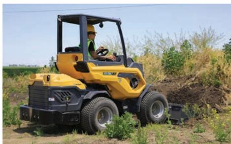
**FOUR-WHEEL DRIVE HYDROSTATIC DIRECT DRIVE MOTORS.** As each wheel has a hydrostatic direct drive motor, hydraulic oil can flow freely to each wheel as needed during transport which helps reduce ground disturbance on turf when making turns. The four-wheel drive hydrostatic direct drive motors also allow for the use of the DBS and torque divider to increase tractive effort in difficult conditions.
