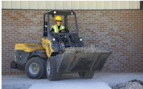
**FRONT-SEATED ARTICULATION.** Front-seated articulation helps the machine work in compact jobsites while keeping turf disturbance a priority.
