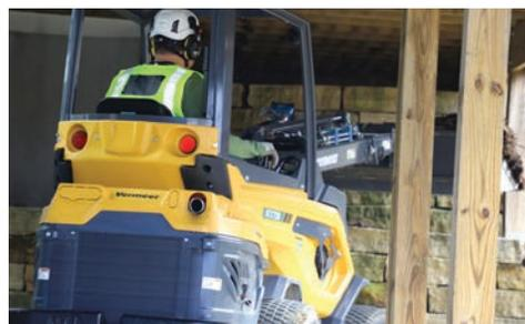
**COMPACT SIZE.** With narrow tires, the ATX720 is 44.5-in (113-cm) wide, while the wider tires make the machine 50.4-in (128-cm) wide. The standard tire configuration allows the ATX720 to fit through a standard 4-ft (1.21-m) gate for backyard access on landscape jobs.
