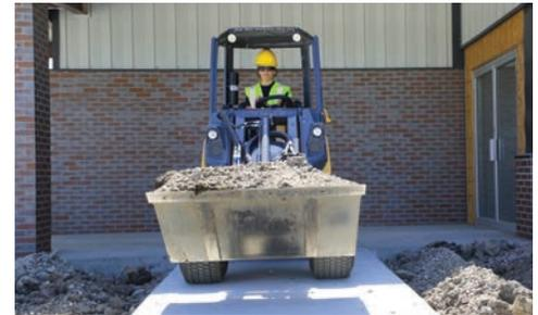
**LIFT-CAPACITY-TO-WEIGHT RATIO.** The ATX720 has a rated operating capacity of 2,155 lb (978 kg) while having a standard weight of 3,549 lb (1,610 kg). This lift-capacity-to-weight ratio allows contractors to use a light machine while still being able to carry heavy materials on the jobsite.
