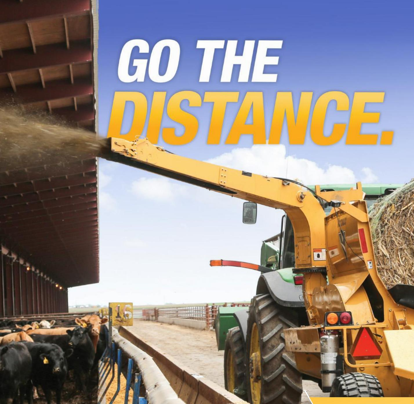
The Vermeer Catapult® CPX9000 bale processor gives operators the ability to process and distribute forage materials consistently and accurately at long distances (up to 100 ft [30.5 m]) – making it ideal for livestock bedding and erosion control applications. It also has the versatility to adjust throw distances and control how the spout is angled to properly distribute the material. However you process it, wherever you put it – this bale processor is built to go the distance.
