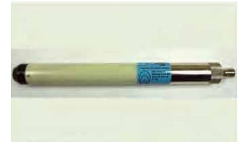
**MINI PROBE (OPTIONS).** Small waterproof transmitter emits a signal that is traced by the receiver, enabling location and depth of non-metallic pipe. Available frequencies: 38 kHz/512 Hz.
