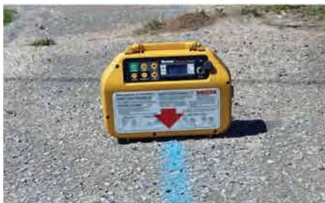
**STRONG INDUCTIVE CAPABILITIES.** For quick verification of utilities for vacuum excavation.
