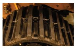
QUAD TRACK SYSTEM. The guad track system offers improved flotation, reduced surface damage and increased tractive effort. Four-wheel steer and crab steering are functional with both quad track and rubber tire options.
