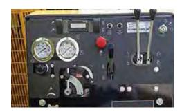
**CONTROL PANEL.** Allows for infinite hydraulic control of bit speed, rotation and travel. Two hydraulic gauges show the operator the down-force pressure and bit rpm. The dual-speed motor allows for a greater speed range, supporting various bit diameters and surface conditions.
