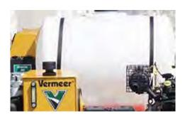
WATER SYSTEM. 100-gal (379-L) available for cooling bit with variable flow from up to 2.8 gpm (10.6 L/min).
