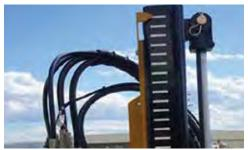
MAST WITH DEPTH GAUGE. Bit travel range of 24 in (61 cm) of vertical movement. Keep track of jobsite progress with depth gauge.
