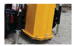
**LEVELING JACKS.** Dual jacks allow for vertical placement of a bit featuring a level located on the front of the machine for precise positioning.
