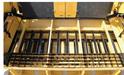
**SELF-CLEANING TANK.** Slats wipe the 2000 gal (7570.8 L) bottom clean as they move material.
