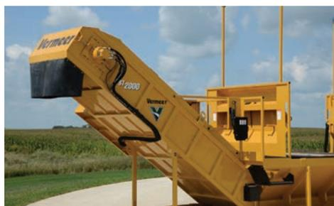
**GENEROUS DISCHARGE CLEARANCE.** 84" (213.4 cm) discharge height allows for multiple loading options.
