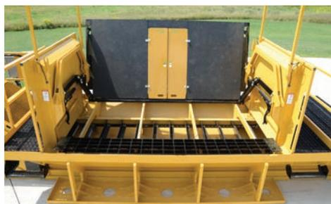
**SWING-OPEN HATCH.** Open access to tank ensures fast and reliable unloading while minimizing splatter for a tidy jobsite.
