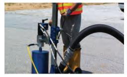
COMPACT CORE DRILL (OPTION). The Compact Core Drill allows vacuum excavation to be performed in areas where pavement or asphalt must be removed prior to potholing by cutting a uniform hole into the pavement. Its patented vacuum suction base keeps it securely in place while the hydraulic pump powers the drill. The Compact Core Drill is capable of cutting holes 6 in, 8 in or 10 in (15.2 cm, 20.3 cm or 25.4 cm) in diameter.
