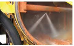
IN-TANK WASH-DOWN. Delivers a high-pressure water spray to the tank interior helping simultaneously dump material and clean the inside of the tank. Minimizes clean up time and helps remove difficult debris.
