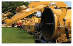
CAM-OVER REAR DOOR. Provides a 360-degree positive seal, even under reverse pressure without additional clamping requirements. The highly reliable cam-over door has a no in-tank moving parts, so all maintenance is external.
