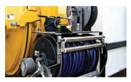
SEWER JETTER (OPTION). The Sewer Jetter system turns your Vermeer vacuum system into a versatile jetter/vac combination unit. It is available with 12 gpm @ 3,000 psi or 18 gpm @ 2,000 psi with 500 ft (152 m) x 1/2 in (1.3 cm) jetter hose.
