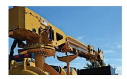
HYDRAULIC BOOM (OPTION). 4 ft or 5 ft (10.2 cm or 12.7 cm) Exclusive telescoping boom maintains hose length during extension and incorporates a remote controlled hydraulic valve for vacuum shut off. Available with manual or hydraulic rotations.
