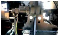
OMSI GEARBOX. OMSI air-shift transfer case is a proven design used throughout the industry to provide the power of the engine to all vacuum components for maximum efficiency and power.
