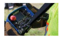
**FULL-FUNCTION, WIRELESS CAN BUS CONTROLS.** The radio remote monitors and controls all machine functions and vital information. Remote straps to the operator and features a machine stop.
