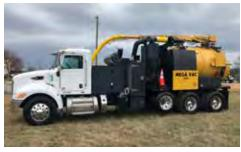
LIGHTWEIGHT. One of the lightest 8-cu yd3 (6.1-cu m³) trucks in the industry to maximize payload. Optional air weigh scale available to monitor live weight of the truck and payload.
