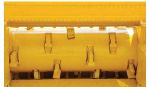
**DUPLEX DRUM.** The patented Series II duplex drum system improves cutting performance, and reversible hammers and tips simplify maintenance and nearly double wear life.
