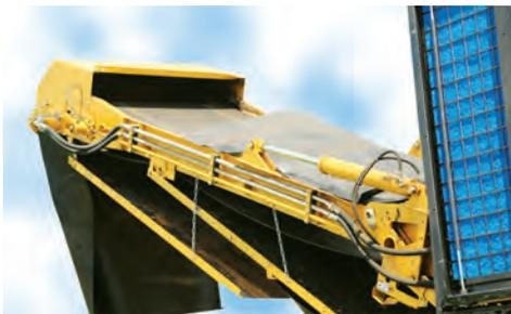
**LOADOUT CONVEYOR.** A smooth discharge conveyor belt, equipped with a scraper that cleans the belt as it passes back to the mill box, reduces material buildup on the belt. Dual chutes help to separate shingle dust from nails.
