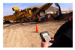
**RESPONSIVE MACHINE.** When a contaminant is detected, Damage Defense system idles the engine down, reverses the infeed or tub, and disengages the clutch.
