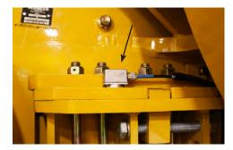
**VERMEER EXCLUSIVE.** Damage Defense system uses exclusive technology to sense metal vibration in the infeed to help prevent major machine damage.
