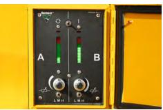
JOBSITE SPECIFIC. Sensitivity settings can be adjusted for specific jobsite conditions to help reduce nuisance shutdowns.
