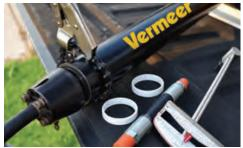
**LONG-LASTING PERFORMANCE.** Wear rings on pistons help extend tool life and maximize tool performance.
