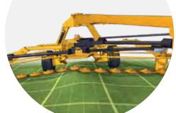
3 The hydraulic suspension system works in conjunction with the split cutter bar to reduce cutter bar weight on the ground, increase flex and allow the TM1200 to follow ground contour.
