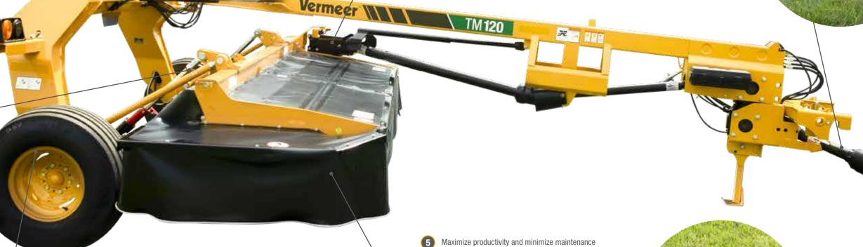
time with a heavy-duty, modular, shaft-driven cutter bar. Not only is it backed by the Vermeer 3-year cutter bar coverage, but two features make it quick and convenient to replace key components — the Quick-Clip® blade retention system and Quick-Change™ shear ring. Get back up and mowing in the field.
