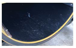
**POLYMER LINER.** The polymer liner inside the debris tank on the bottom half makes for ease of dumping and cleanout.
