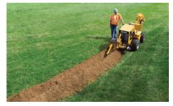
SET YOUR SPEED. The electronic control allows for convenient setting of the creep speed to help optimize performance on longer distance installations, allowing productivity while helping to reduce operator fatigue, whether trenching or plowing.
