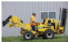
ATTACHMENTS FOR THE JOB. The PTX42 has a variety of versatile attachment options, including a backhoe, trencher, plow, porta bore and two reel carriers. Select the right attachment that best fits the needs of your operation and jobsite.
