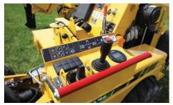
HANDS-ON CONTROL. The PTX42 plow/trencher offers walk-beside hand controls that pivot from side to side of the machine for convenient operation and to maneuver around potential obstacles or congested spaces on a jobsite. The control placement can help minimize operator reach and maintain operator comfort.
