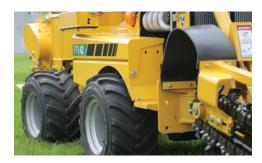
STAY ON TRACK. For varying ground conditions, choose from tires or tracks - the PTX42 offers a 23" (58.4 cm) foam-filled tire option, while the slightly larger 26" (66 cm) air-filled tires can help with traction. A 23" (58.4 cm) dual air-filled tire option offers stability and lower ground pressure, and a track option is well-suited for uneven terrain.
