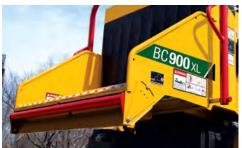
**OPERATOR SAFETY.** Combined with the patented bottom feed stop bar is the four-position upper feed stop bar with dual stop positions and forward/reverse feed positions. Mounted over the feed table, it enables the operator to stop the feed rollers and select forward or reverse operations. Dual reset/hold-to-run buttons allow the operator to readily reset the bottom feed stop bar.
