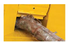
LARGE RECTANGULAR FEED OPENING. The large 9 in x 14 in (22.9 cm x 35.6 cm) feed opening helps boost productivity by reducing the need to trim heavily branched material before feeding it into the chipper.
