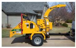
**EASE OF SERVICE.** This machine offers direct access to all parts of the chipper for routine maintenance without having to remove any shields. A dripless oil filter and five grease points are provided to reduce work effort and speed up service time.
