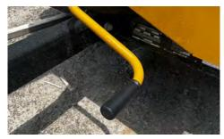
MANUAL CLUTCH. Manual clutch engagement transfers belt tension from the disk to the engine smoothly to help prevent premature wear.
