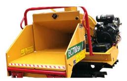
**BOTTOM FEED STOP BAR.** Is strategically located to make it possible for an operator to strike the bar and shut off the feed mechanism.
