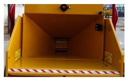
**LARGE INFEED OPENING.** 6 in x 8 in (15.2 cm x 20.3 cm) makes feeding irregular material efficient and minimizes the amount of saw cuts needed prior to feeding the chipper.
