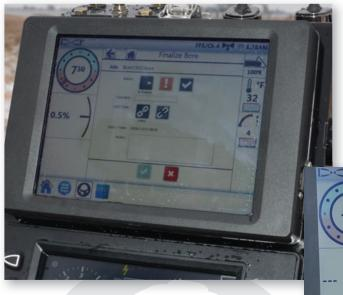
BoreAssist is a user-friendly application that helps the drill operator load and review the bore plan on the machine, then follow the rod-by-rod plan, make changes, add obstacles and utilities, define a reamer diameter and radius around bore plan... or even design a simple bore plan on the rig.
