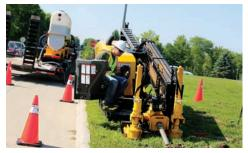
**RIGHT POWER, RIGHT FOOTPRINT.** The D20x22 S3 offers a sizeable increase in power and rotational torque over its predecessor, the D16x20 Series II, making it well-suited to install cable, fiber and product pipe efficiently and productively.
